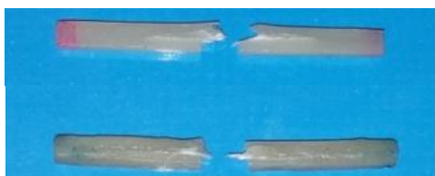
Fig. 20. The fracture pattern of FRC with braided glass (groups B2, D2)
