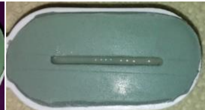
Fig. 15. First layer of composite with 0.9 mm thickness
