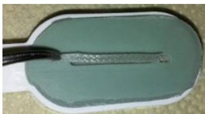
Fig. 16. Placing of the fibre on the first layer of composite and light curing for 60 seconds
