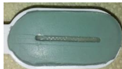
Fig. 16. Placing of the fibre on the first layer of composite and light curing for 60 seconds
