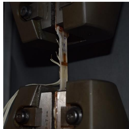
Fig. 27. The positioning of the test specimen between the machine's wedge grips
