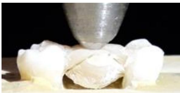
Fig. 51. Fracture pattern for parallel design of the fibres
