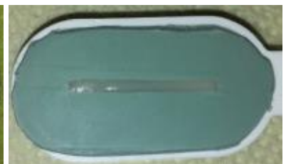
Fig. 17. Placing the second layer of composite and light curing for 60 seconds
