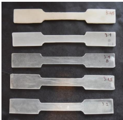
Fig. 23. Test specimens from acrylic resin corresponding to the five groups
