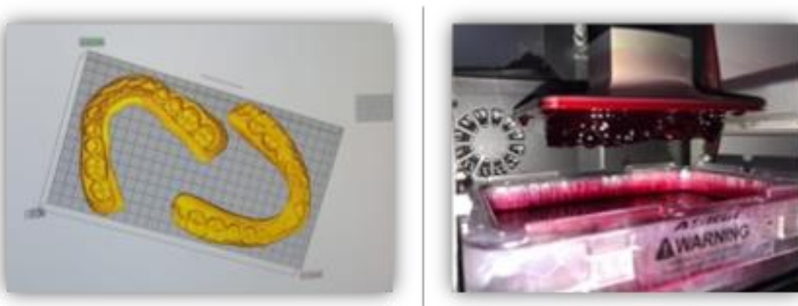
Figure 13. The 3D-printed models: from STL files to printed models.
