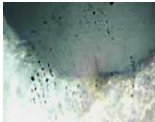
Figure 75. The aspect of interface at the level of the ceramic restoration fixed with Meron Plus after the immersion in 20% acid citric
