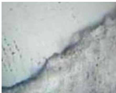
Figure 79. The interface between the ceramic restoration and the Variolik N resin after the immersion in artificial saliva
