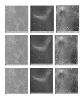
**Figure 2.** SEM images of the composite surface at 500× magnification: **(A)** GrandioSO; **(B)** Clearfil Majesty ES flow, and **(C)** G-aenial Flo X
