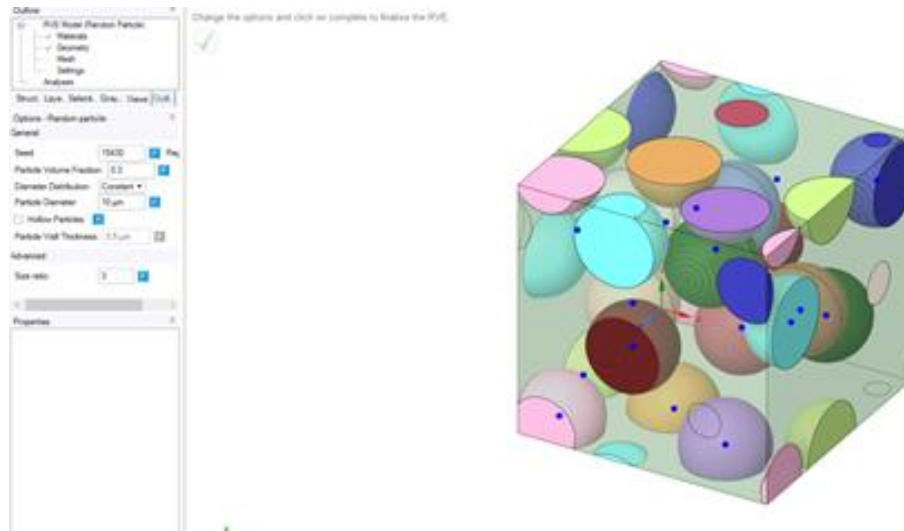
Fig.97 Material designer setup related graphical representations of the: 3D view of the random particle type of arrangement
