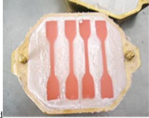
Fig.8d. Introduction of the resin in the mold
