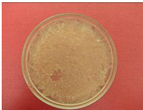
Fig.43 - Microbial load of sample P1 after processing with brushes and polishing paste that had been used before (dilution 10^{-3} )
