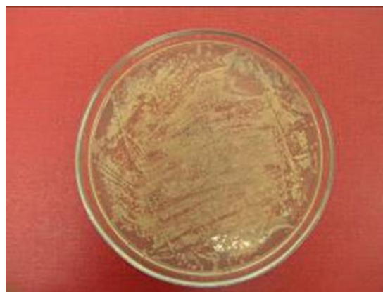
Fig.49 - Microbial load of sample P3 after processing with brushes and polishing paste that had been used before (dilution 10^{-3} )
