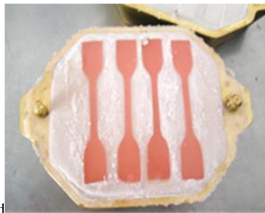
Fig.8d. Introduction of the resin in the mold
