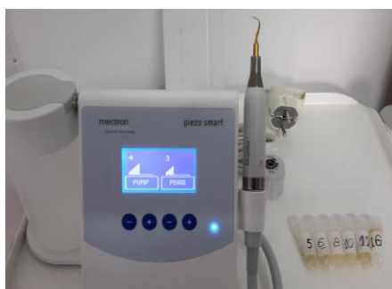
Figure II.5. The ultrasonic piezoelectric system, together with the instrumented samples
