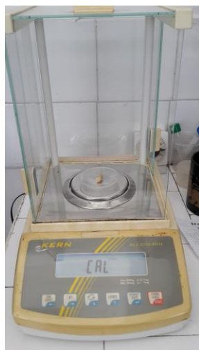
Figure II.7. The scale used for the weight measurements before and after the instrumentation
