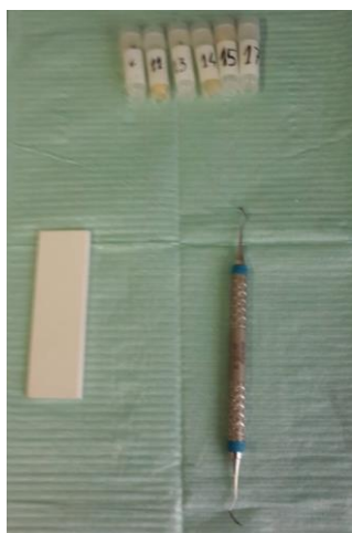
Figure II.4. The Gracey curette 5/6, together with the instrumented samples and the Arkansas stone
