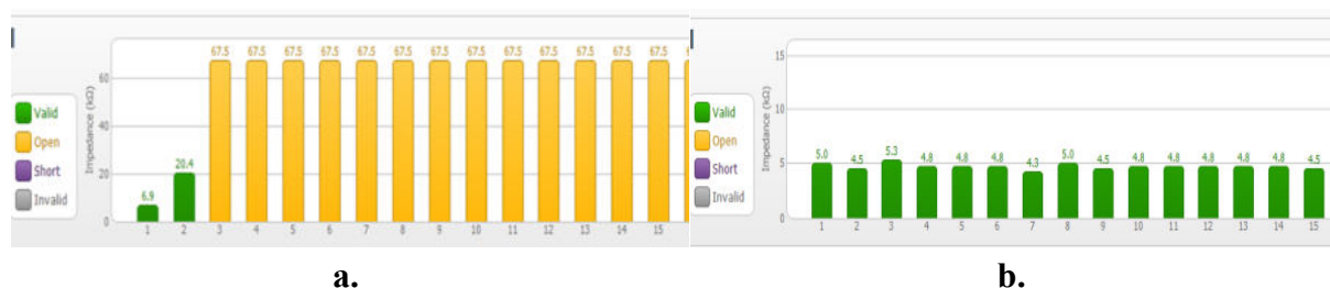
Fig. I.2-5.10. Impedances values measured intraoperatively (a) and at the activation time (b)
