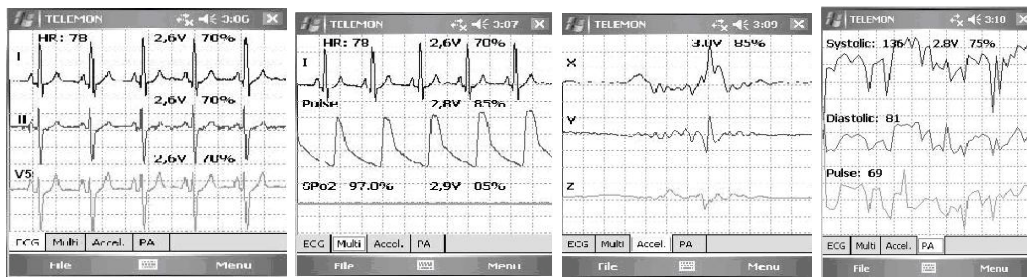
Figure 12: The Personal server interface: (a) 3 ECG traces, (b) one ECG trace, pulse waveform and SpO2, (c) 3 accelerometer traces, (d) systolic and diastolic pressure from BPM
